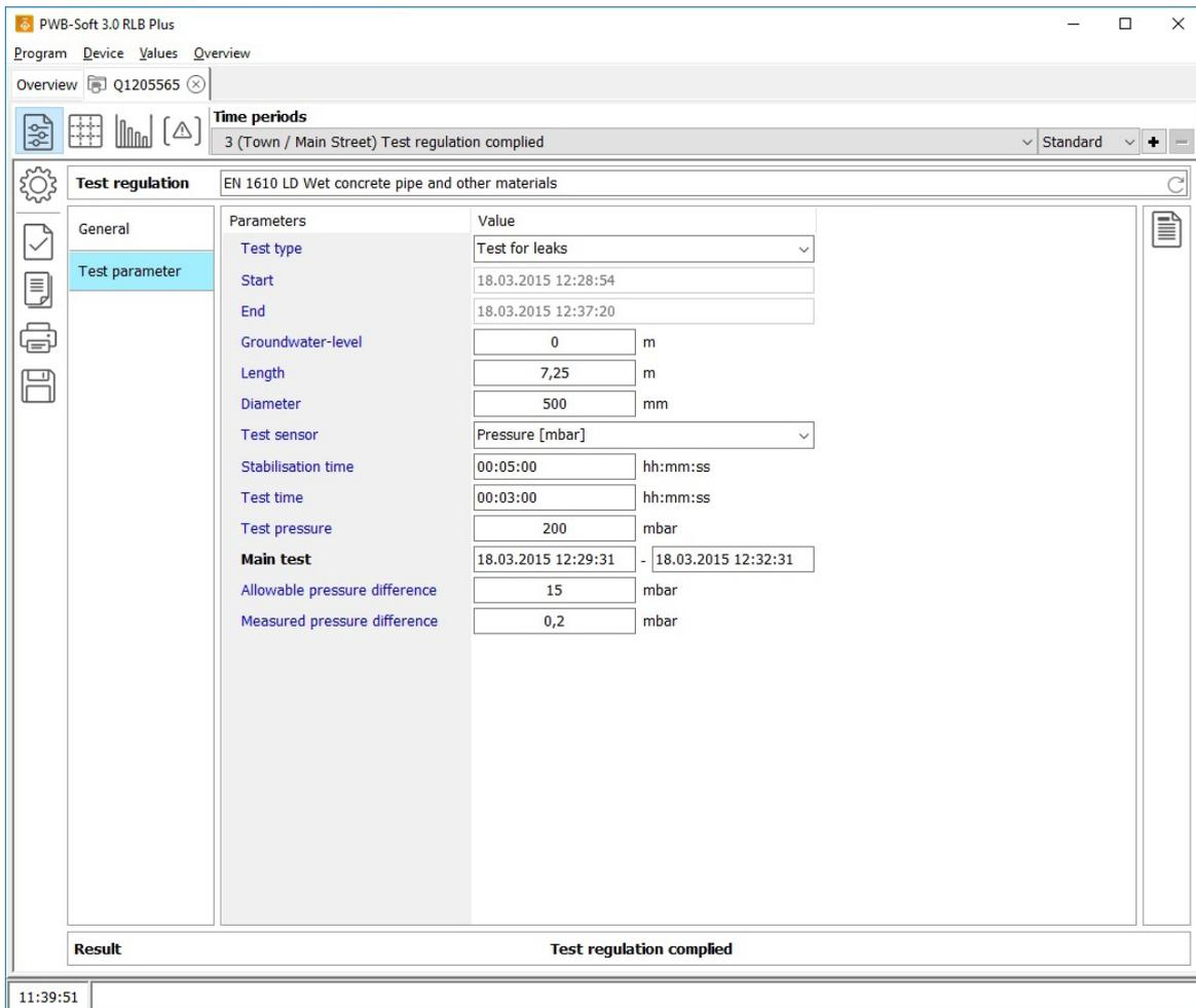
The screenshot shows the PWB-Soft 3.0 RLB Plus software interface. The main window displays the 'Test regulation' section for 'EN 1610 LD Wet concrete pipe and other materials'. The 'Test parameter' tab is active, showing a table of parameters and their values.
