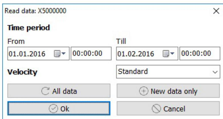
The dialog on reading the device shows the found data range. Clicking on „OK“ starts reading the data of the shown period. The period can also be restricted to read part of the saved data only. You will find further information in chapter „5 Reading and restarting data logger“.
