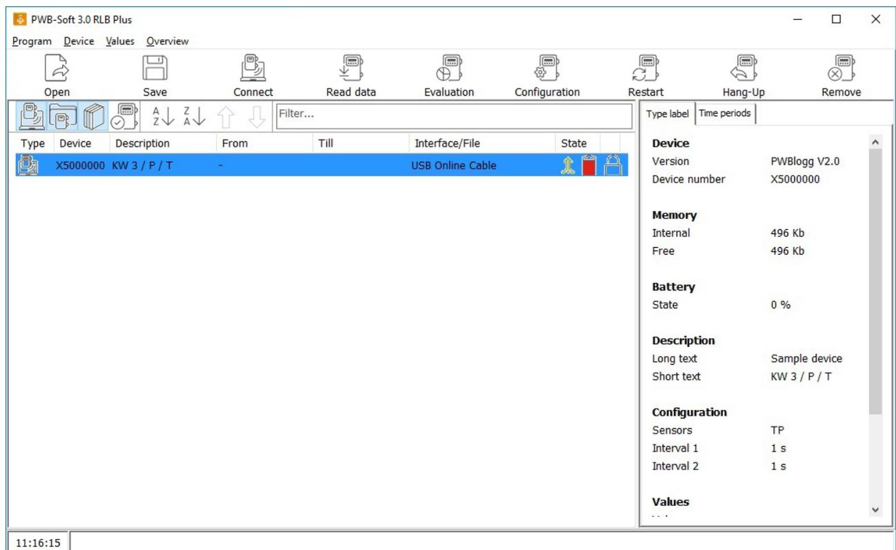
A double click on this LED symbol or using the menu function „Device“ → „Hang-Up“ separates the connection. Thereby the serial interface will be closed. The device itself remains in the list. If applicable, the already read data can be evaluated further. „Device“ → „Reconnect“ calls the connection to the device again. Thereby status information and parameters will be newly imported.
