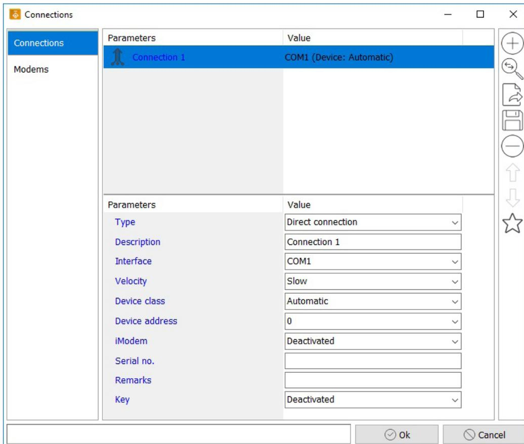
Initially, an entry for the USB online cable must be made. Leave the other settings unchanged for the time being.
