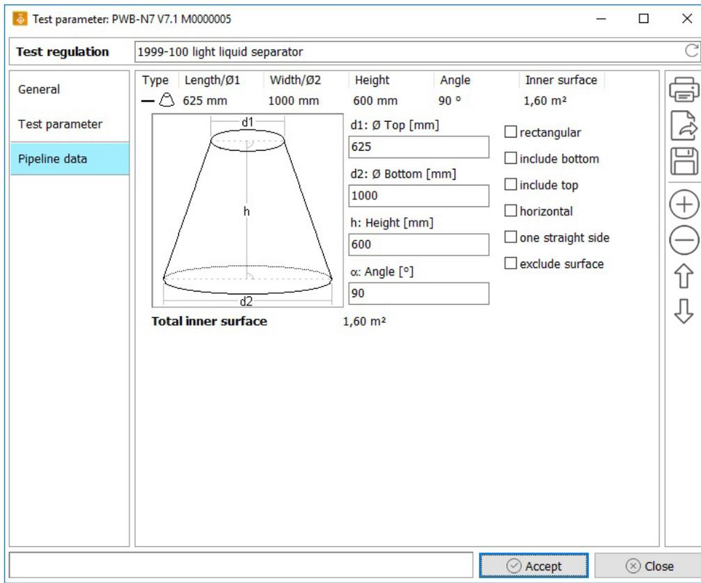
Individual parts of the test object are specified in the list. Thus defined, the order in the list corresponds to the real body of the object, that is, the first/on top entry corresponds to the top part of the object. The buttons  $\uparrow$  and  $\downarrow$  are used to facilitate moving individual parts in their sequential arrangement and hence the layout of the test object. The button  $+$  allows including a further part and  $-$  removes the highlighted entry from the list.
