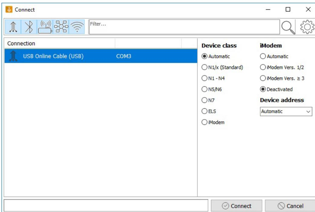
Initially, the chosen connection dialog will appear showing important defaults which can be specified again and adapted. Changes made here become defaults for the next connecting attempt.
