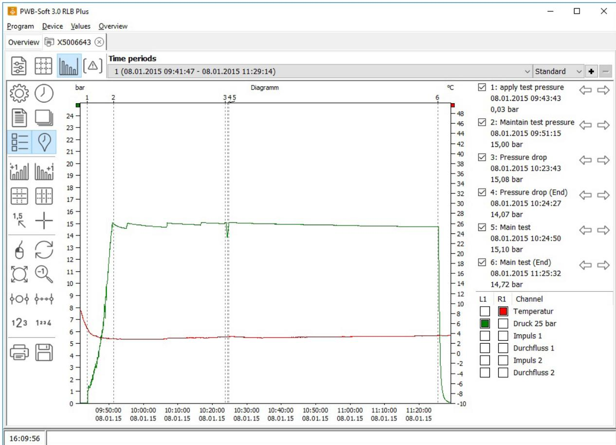
For that purpose, marks will be sequentially superimposed and moved to the correct position by right mouse button. The arrow keys next to the mask can be used for fine-tuning. The section can also be enlarged by the zoom function.
