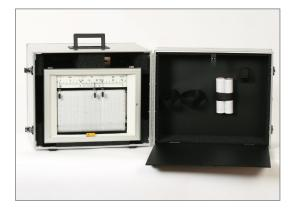
Connecting conditions strip chart recorder for indicator pressure, thread G 1/2B backward or downward strip chart recorder for indicator temperature, sensor type as remote sensor with union nut or smooth sensor, sensor length 100 mm at least, brass, steel or stainless steel thermowell.
