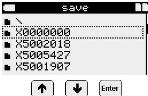
The line „\`“` refers to the root directory of the MMC/SD. This is only provided when saving data to be able to select the root directory purposefully. So, when loading or opening files, there can already be file names visible instead.
