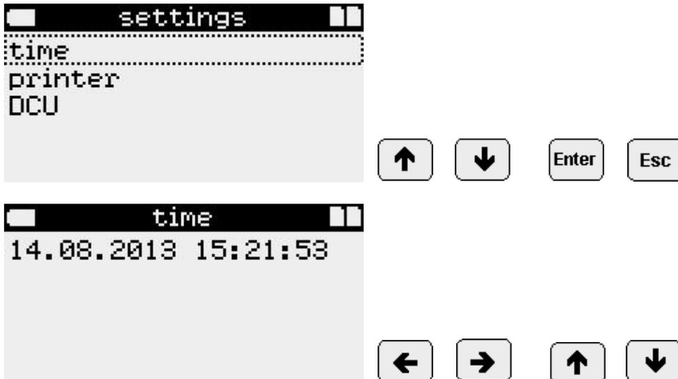
Setting digits is done by arrow keys. The arrow keys left/right are used for selecting a digit. The arrow keys up/down alter a digit. Only valid data and times can be entered. Instead of manual input, the time can also be set by taking from a data logger using *connect*. If there is a power failure (battery change), time will get lost.
